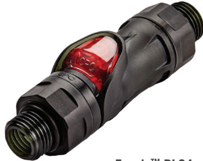
Everis™ PLQ4 Nominal flow of 1/4" (6.4 mm) with a Cv of 1.3 (Kv 1.1) Termination options: hose barb, locking hose barb, SAE, G thread
