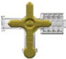
FCHPFFMR-003 3-Way High Pressure Stopcock, Female Luer to Female Luer to Male Luer with Luer Lock Ring, Clear Polycarbonate Body and Lock Ring, 4-Arrow Gold Color Acetal Diverter
