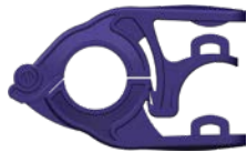
CPAN75 (-U71, -U75, -U706) Tri-Clover Easy-Open Clamp for Mini Flange, .5" (12.7 mm) to .75" (19.0 mm), Glass-Reinforced White, Blue, or Orange Nylon
