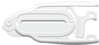
CPT90 (-U71, -U706) PharmaLok™ Small and Thin-Walled Tube Clamp, Wall Thickness 1/32" (0.79 mm) to 3/32" (2.4 mm), Max OD 1/2" (12.7 mm), Glass-Filled White or Orange Nylon
