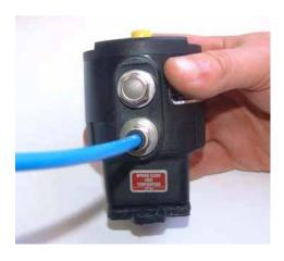
**8.** Attach the actuator to the valve body; insert the retaining fasteners.
