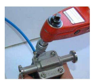
This ensures that the diaphragm correctly seats before further tightening.
