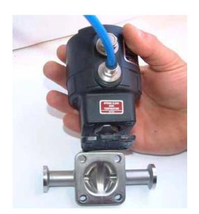
**5.** Remove diaphragm from actuator by turning anti-clockwise.
